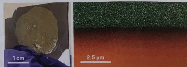
A new electrochemical process puts semiconductors at researchers' fingertips (left). The process creates germanium thin films (green) on silicon (orange) with specks of gallium (white), as shown by electron microscopy and X-ray analysis (right).
